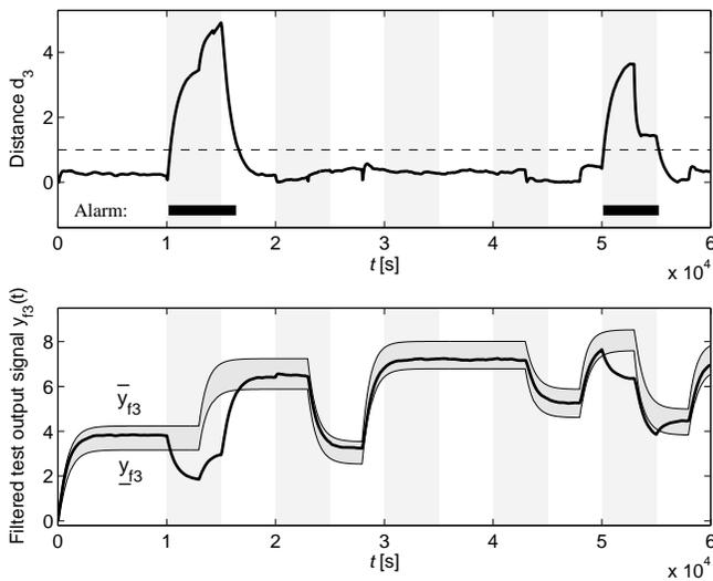
Fig. 9. Results of the fault detection with INFUMO3
