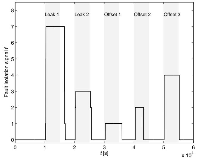
Fig. 10. Results of the fault isolation with a bank of INFUMOs
