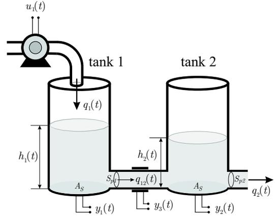
Fig. 2. Two-tank laboratory plant
