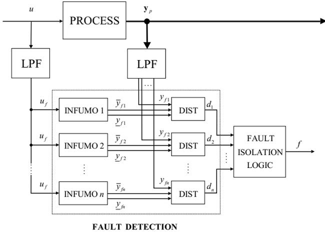
Fig. 1. Fault-isolation system using INFUMO models for FD
